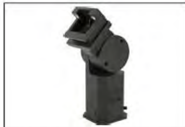
Slipfitter Mount An optional cast aluminum mast arm adapter secures fixture head to nominal 2"(2-3/8"O.D. pipe size) horizontal steel tenon arm.
