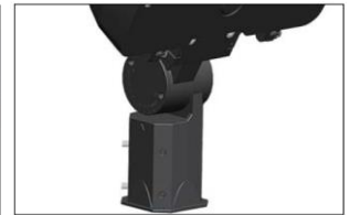
Slipfitter Mount An optional cast aluminum mast arm adapter secures fixture head to nominal 2" (2-3/8" O.D. pipe size) horizontal steel tenon arm.
